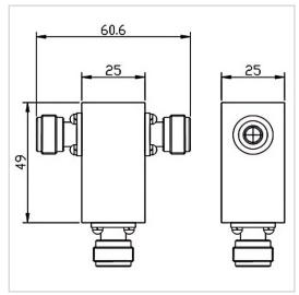
RF Solution offer a wide selection of 2 Ways Power Divider for global customers. PD02-F6149-N-5-6GHz is a 2 Ways Power Divider in Frequency Range of 5.0~6.0 GHz. It is made of high quality materials under a high standard, the Insertion Loss Max of this product is 0.8 dB, Isolation Min is 20 dB and Split Loss is 3.5 dB. The component has a good working performance and stability, it is ideal for handling a Rated Power of 300 W.
