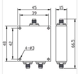
RF Solution offer a wide selection of 2 Ways Power Divider for global customers. PD02-F4548-S-698-3800MHz is a 2 Ways Power Divider in Frequency Range of 698~3800 MHz. It is made of high quality materials under a high standard, the Split Loss of this product is 3.0 dB, Insertion Loss Max is 0.8 dB and Isolation Min is 20.0 dB. The component has a good working performance and stability, it is ideal for handling a Rated Power of 50 W.
