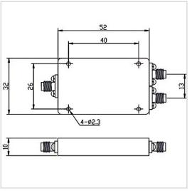
RF Solution offer a wide selection of 2 Ways Power Divider for global customers. PD02-F3252-S-0.5-6GHz is a 2 Ways Power Divider in Frequency Range of  $0.5\sim6.0$  GHz. It is made of high quality materials under a high standard, the Insertion Loss Max of this product is 1.0 dB, Isolation Min is 20.0 dB and Amplitude Unbalance is  $\pm0.3$  dB. The component has a good working performance and stability, it is ideal for handling a Forward Power of 30 W.
