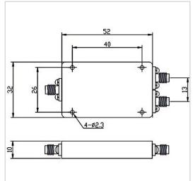
RF Solution offer a wide selection of 2 Ways Power Divider for global customers. PD02-F3252-S-0.5-4GHz is a 2 Ways Power Divider in Frequency Range of  $0.5\sim4.0$  GHz. It is made of high quality materials under a high standard, the Insertion Loss Max of this product is 0.5 dB, Isolation Min is 20.0 dB and Amplitude Unbalance is  $\pm 0.2$  dB. The component has a good working performance and stability, it is ideal for handling a Forward Power of 30 W.
