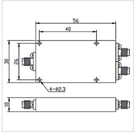
RF Solution offer a wide selection of 2 Ways Power Divider for global customers. PD02-F3056-S-0.5-8GHz is a 2 Ways Power Divider in Frequency Range of  $0.5{\sim}8.0$  GHz. It is made of high quality materials under a high standard, the Insertion Loss Max of this product is 1.5 dB, Isolation Min is 20.0 dB and Amplitude Unbalance is  $\pm 0.3$  dB. The component has a good working performance and stability, it is ideal for handling a Forward Power of 30 W.
