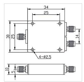
RF Solution offer a wide selection of 2 Ways Power Divider for global customers. PD02-F3034-S-2-4GHz is a 2 Ways Power Divider in Frequency Range of 2.0~4.0 GHz. It is made of high quality materials under a high standard, the Insertion Loss Max of this product is 0.4 dB, Isolation Min is 20 dB and Amplitude Unbalance is  $\pm$ 0.2 dB. The component has a good working performance and stability, it is ideal for handling a Forward Power of 30 W.
