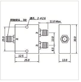
RF Solution offer a wide selection of 2 Ways Power Divider for global customers. PD02-F3025-S-90-110MHz is a 2 Ways Power Divider in Frequency Range of  $90\sim110$  MHz. It is made of high quality materials under a high standard, the Insertion Loss Max of this product is 0.65 dB, Isolation Min is 20.0 dB and Amplitude Balance is  $\pm0.2$  dB. The component has a good working performance and stability, it is ideal for handling a Rated Power of 1 W.
