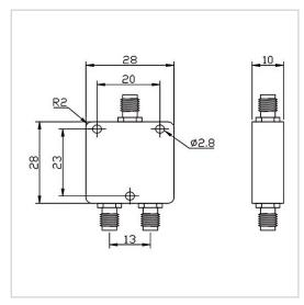
RF Solution offer a wide selection of 2 Ways Power Divider for global customers. PD02-F2828-S-DC-6GHz is a 2 Ways Power Divider in Frequency Range of DC $\sim$ 6.0 GHz. It is made of high quality materials under a high standard, the Insertion Loss Max of this product is 7.0( $\pm$  0.4) dB, Isolation Min is 6.0 dB and VSWR Max is 1.25. The component has a good working performance and stability, it is ideal for handling a Rated Power of 2 W.
