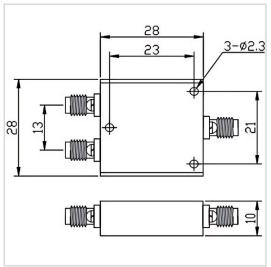
RF Solution offer a wide selection of 2 Ways Power 3-\$\phi\_{2.3}\$ Divider for global customers. PD02-F2828-S-1-4GHz is a 2 Ways Power Divider in Frequency Range of 1.0~4.0 GHz. It is made of high quality materials under a high standard, the Insertion Loss Max of this product is 0.5 dB, Isolation Min is 20 dB and Amplitude Unbalance is ±0.3 dB. The component has a good working performance and stability, it is ideal for handling a Forward Power of 30 W.
