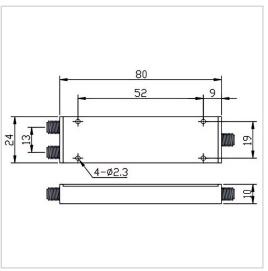
RF Solution offer a wide selection of 2 Ways Power Divider for global customers. PD02-F2480-S-1-12.4GHz is a 2 Ways Power Divider in Frequency Range of  $1.0 \sim 12.4$  GHz. It is made of high quality materials under a high standard, the Insertion Loss Max of this product is 1.5 dB, Isolation Min is 16 dB and Amplitude Unbalance is  $\pm 0.4$  dB. The component has a good working performance and stability, it is ideal for handling a Forward Power of 20 W.
