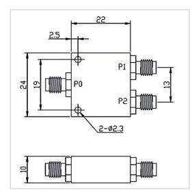
RF Solution offer a wide selection of 2 Ways Power Divider for global customers. PD02-F2422-S-10-1000MHz is a 2 Ways Power Divider in Frequency Range of 10~1000 MHz. It is made of high quality materials under a high standard, the Amplitude Balance of this product is ±0.5 dB, Insertion Loss Max is 1.0 dB and Isolation Min is 20.0 dB. The component has a good working performance and stability, it is ideal for handling a Forward Power of 1 W.
