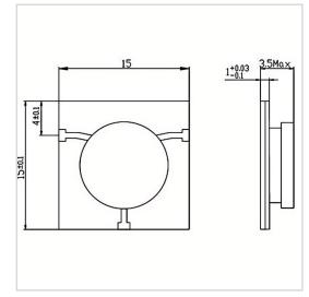
RF Solution offer a wide selection of Microstrip Circulator for global customers. MH1515-10 is a Microstrip Circulator in Frequency Range of 2.0~6.0 GHz. It is made of high quality materials under a high standard, the Bandwidth Max of this product is 100%, Insertion Loss Max is 1.50 dB and Isolation Min is 10.0 dB. The component has a good working performance and stability, it is ideal for handling a Forward Power of 50 W.
