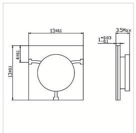
RF Solution offer a wide selection of Microstrip Circulator for global customers. MH1313-10 is a Microstrip Circulator in Frequency Range of 2.7~6.2 GHz. It is made of high quality materials under a high standard, the Bandwidth Max of this product is 66%, Insertion Loss Max is 1.20 dB and Isolation Min is 13.0 dB. The component has a good working performance and stability, it is ideal for handling a Forward Power of 50 W.
