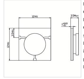
RF Solution offer a wide selection of Microstrip Circulator for global customers. MH1212-10 is a Microstrip Circulator in Frequency Range of 2.7~8.0 GHz. It is made of high quality materials under a high standard, the Bandwidth Max of this product is 100%, Insertion Loss Max is 0.40~0.80 dB and Isolation Min is 14.0~20.0 dB. The component has a good working performance and stability, it is ideal for handling a Forward Power of 50 W.
