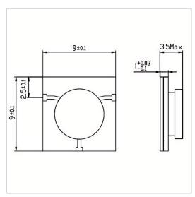
RF Solution offer a wide selection of Microstrip Circulator for global customers. MH0909-10 is a Microstrip Circulator in Frequency Range of  $5.0 \sim 7.0$  GHz. It is made of high quality materials under a high standard, the Bandwidth Max of this product is 18%, Insertion Loss Max is 0.40 dB and Isolation Min is 20.0 dB. The component has a good working performance and stability, it is ideal for handling a Forward Power of 50 W.
