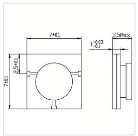
RF Solution offer a wide selection of Microstrip Circulator for global customers. MH0707-10 is a Microstrip Circulator in Frequency Range of 5.0~13.0 GHz. It is made of high quality materials under a high standard, the Bandwidth Max of this product is 100%, Insertion Loss Max is 1.20 dB and Isolation Min is 11.0 dB. The component has a good working performance and stability, it is ideal for handling a Forward Power of 50 W.
