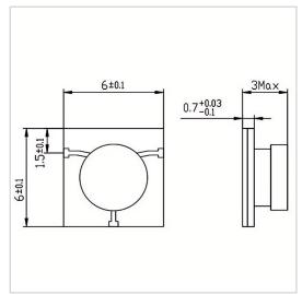
RF Solution offer a wide selection of Microstrip Circulator for global customers. MH0606-07 is a Microstrip Circulator in Frequency Range of 7.0~13.0 GHz. It is made of high quality materials under a high standard, the Bandwidth Max of this product is 20%, Insertion Loss Max is 0.40~0.80 dB and Isolation Min is 15.0~20 dB. The component has a good working performance and stability, it is ideal for handling a Forward Power of 50 W.
