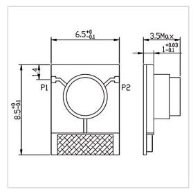
RF Solution offer a wide selection of Microstrip Isolator for global customers. MG6585-10 is a Microstrip Isolator in Frequency Range of 5.0~12.0 GHz. It is made of high quality materials under a high standard, the Insertion Loss Max of this product is 0.60 dB, Isolation Min is 16.0 dB and VSWR Max is 1.40. The component has a good working performance and stability, it is ideal for handling a Forward Power of 50 W.
