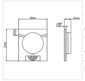
RF Solution offer a wide selection of Microstrip Isolator for global customers. MG1517-10 is a Microstrip Isolator in Frequency Range of 2.0~6.0 GHz. It is made of high quality materials under a high standard, the Insertion Loss Max of this product is 1.30~1.50 dB, Isolation Min is 10.0~11.0 dB and VSWR Max is 1.70~1.80. The component has a good working performance and stability, it is ideal for handling a Forward Power of 50 W.
