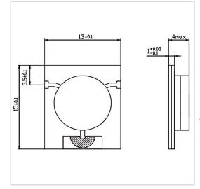
RF Solution offer a wide selection of Microstrip Isolator for global customers. MG1315-10 is a Microstrip Isolator in Frequency Range of 2.7~6.2 GHz. It is made of high quality materials under a high standard, the Insertion Loss Max of this product is 1.00~1.20 dB, Isolation Min is 13.0~15.0 dB and VSWR Max is 1.50~1.60. The component has a good working performance and stability, it is ideal for handling a Forward Power of 50 W.
