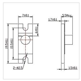
RF Solution offer a wide selection of Microstrip Isolator for global customers. MG0719-15 is a Microstrip Isolator in Frequency Range of 9.0~10.5 GHz. It is made of high quality materials under a high standard, the Insertion Loss Max of this product is 0.60 dB, Isolation Min is 18.0 dB and VSWR Max is 1.30. The component has a good working performance and stability, it is ideal for handling a Forward Power of 10 W.
