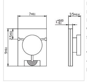
RF Solution offer a wide selection of Microstrip Isolator for global customers. MG0709-10 is a Microstrip Isolator in Frequency Range of 5.0~13.0 GHz. It is made of high quality materials under a high standard, the Insertion Loss Max of this product is 1.00~1.20 dB, Isolation Min is 11.0~13.0 dB and VSWR Max is 1.60~1.70. The component has a good working performance and stability, it is ideal for handling a Forward Power of 50 W.
