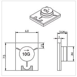
RF Solution offer a wide selection of Microstrip Isolator for global customers. MG0675-10 is a Microstrip Isolator in Frequency Range of 5.0~12.0 GHz. It is made of high quality materials under a high standard, the Insertion Loss Max of this product is 0.60 dB, Isolation Min is 16.0 dB and VSWR Max is 1.35. The component has a good working performance and stability, it is ideal for handling a Forward Power of 5 W.
