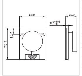
RF Solution offer a wide selection of Microstrip Isolator for global customers. MG0675-07 is a Microstrip Isolator in Frequency Range of 5.0~13.0 GHz. It is made of high quality materials under a high standard, the Insertion Loss Max of this product is 0.40~0.80 dB, Isolation Min is 15.0~20.0 dB and VSWR Max is 1.20~1.45. The component has a good working performance and stability, it is ideal for handling a Forward Power of 50 W.
