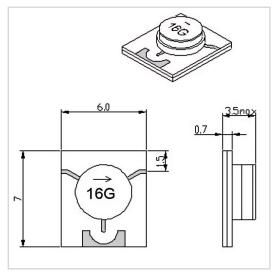
RF Solution offer a wide selection of Microstrip Isolator for global customers. MG0607-07-X-15.0-17.0GHz is a Microstrip Isolator in Frequency Range of 15.0~17.0 GHz. It is made of high quality materials under a high standard, the Insertion Loss Max of this product is 0.70 dB, Isolation Min is 15.0 dB and VSWR Max is 1.45. The component has a good working performance and stability, it is ideal for handling a Forward Power of 5 W.
