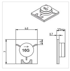
RF Solution offer a wide selection of Microstrip Isolator for global customers. MG0607-07-X-14.5-17.5GHz is a Microstrip Isolator in Frequency Range of 14.5~17.5 GHz. It is made of high quality materials under a high standard, the Insertion Loss Max of this product is 0.70 dB, Isolation Min is 15.0 dB and VSWR Max is 1.45. The component has a good working performance and stability, it is ideal for handling a Forward Power of 5 W.
