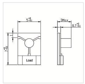
RF Solution offer a wide selection of Microstrip Isolator for global customers. MG0507-07 is a Microstrip Isolator in Frequency Range of 12.7~14.7 GHz. It is made of high quality materials under a high standard, the Insertion Loss Max of this product is 0.60 dB, Isolation Min is 19.0 dB and VSWR Max is 1.30. The component has a good working performance and stability, it is ideal for handling a Forward Power of 4 W.
