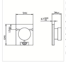
RF Solution offer a wide selection of Microstrip Isolator for global customers. MG0506-07 is a Microstrip Isolator in Frequency Range of 11.0~19.5 GHz. It is made of high quality materials under a high standard, the Insertion Loss Max of this product is 0.50~0.60 dB, Isolation Min is 16.0~20.0 dB and VSWR Max is 1.25~1.45. The component has a good working performance and stability, it is ideal for handling a Forward Power of 20 W.
