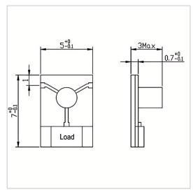
RF Solution offer a wide selection of Microstrip Isolator for global customers. MG0505-07-X-13.75-14.5GHz is a Microstrip Isolator in Frequency Range of 13.75~14.5 GHz. It is made of high quality materials under a high standard, the Insertion Loss Max of this product is 0.50~0.60 dB, Isolation Min is 18.0~20.0 dB and VSWR Max is 1.25~1.30. The component has a good working performance and stability, it is ideal for handling a Forward Power of 10 W.
