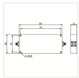
RF Solution offer a wide selection of Low Pass Filter for global customers. LPF-DCM500A-S is a Low Pass Filter in Frequency Range of DC~500 MHz. It is made of high quality materials under a high standard, the Insertion Loss Max of this product is 2.0 dB, Rejection Min is 40dB@600-900MHz and VSWR Max is 1.80. The component has a good working performance and stability, it is ideal for handling a Rated Power of 30 W.
