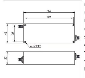
RF Solution offer a wide selection of Low Pass Filter for global customers. LPF-DCM1400A-S is a Low Pass Filter in Frequency Range of DC~1400 MHz. It is made of high quality materials under a high standard, the Insertion Loss Max of this product is 2.0 dB, Rejection Min is 40dB@1484-11000MHz and VSWR Max is 2.00. The component has a good working performance and stability, it is ideal for handling a Rated Power of 20 W.
