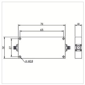
RF Solution offer a wide selection of Low Pass Filter for global customers. LPF-DCM1250A-S is a Low Pass Filter in Frequency Range of DC~1250 MHz. It is made of high quality materials under a high standard, the Insertion Loss Max of this product is 1.0 dB, Rejection Min is 50dB@1560-3300MHz and VSWR Max is 1.50. The component has a good working performance and stability, it is ideal for handling a Rated Power of 40 W.
