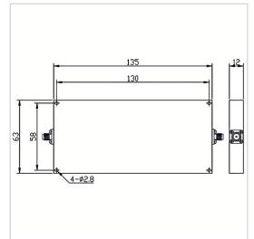
RF Solution offer a wide selection of Low Pass Filter for global customers. LPF-DCM1000A-S is a Low Pass Filter in Frequency Range of DC~1000 MHz. It is made of high quality materials under a high standard, the Insertion Loss Max of this product is 1.5 dB, Rejection Min is 60dB@1230-8000MHz and VSWR Max is 1.80. The component has a good working performance and stability, it is ideal for handling a Rated Power of 20 W.
