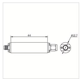
RF Solution offer a wide selection of Low Pass Filter for global customers. LPF-DCG18A-S is a Low Pass Filter in Frequency Range of DC~18000 MHz. It is made of high quality materials under a high standard, the Insertion Loss Max of this product is 0.6 dB, Rejection Min is 25dB@21.6GHz / 50dB@24.3-GHz and VSWR Max is 1.80. The component has a good working performance and stability, it is ideal for handling a Rated Power of 50 W.
