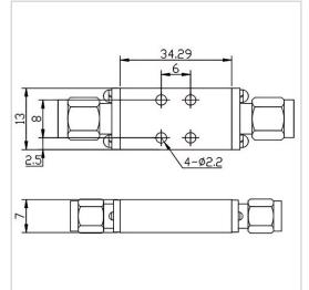
RF Solution offer a wide selection of Low Pass Filter for global customers. LPF-DCG13.6A-S is a Low Pass Filter in Frequency Range of DC~13600 MHz. It is made of high quality materials under a high standard, the Insertion Loss Max of this product is 0.4 dB, Rejection Min is 25dB@22GHz / 40dB@25.5-40GHz and VSWR Max is 1.50. The component has a good working performance and stability, it is ideal for handling a Rated Power of 50 W.
