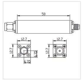
RF Solution offer a wide selection of Low Pass Filter for global customers. LPF-DCG12A-S is a Low Pass Filter in Frequency Range of DC~12000 MHz. It is made of high quality materials under a high standard, the Insertion Loss Max of this product is 0.4 dB, Rejection Min is 25dB@14400 MHz / 55dB@18000 MHz and VSWR Max is 1.70. The component has a good working performance and stability, it is ideal for handling a Rated Power of 50 W.
