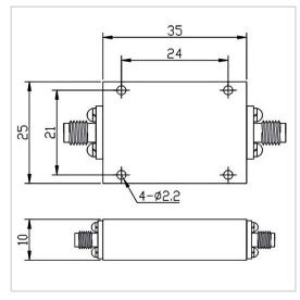
RF Solution offer a wide selection of High Pass Filter for global customers. HPF-5G22A-S is a High Pass Filter in Frequency Range of 5.0~22.0 GHz. It is made of high quality materials under a high standard, the Insertion Loss Max of this product is 2.0dB@5000-5250MHz / 1.0dB@5250-22000MHz, Rejection Min is 60dB@DC-4480MHz and VSWR Max is 1.50. The component has a good working performance and stability, it is ideal for handling a Rated Power of 15 W.
