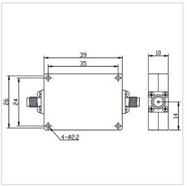
RF Solution offer a wide selection of High Pass Filter for global customers. HPF-4.2G12.75A-S is a High Pass Filter in Frequency Range of 4.20~12.75 GHz. It is made of high quality materials under a high standard, the Insertion Loss Max of this product is 2.00 dB, Rejection Min is 40dB@DC-3.8GHz and VSWR Max is 1.70. The component has a good working performance and stability, it is ideal for handling a Rated Power of 15 W.
