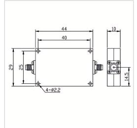
RF Solution offer a wide selection of High Pass Filter for global customers. HPF-3G18A-S is a High Pass Filter in Frequency Range of 3.0~18.0 GHz. It is made of high quality materials under a high standard, the Insertion Loss Max of this product is 2.0dB@3000-3200MHz / 1.4dB@3200-18000MHz, Rejection Min is 40dB@DC-2.7GHz and VSWR Max is 1.67. The component has a good working performance and stability, it is ideal for handling a Rated Power of 15 W.
