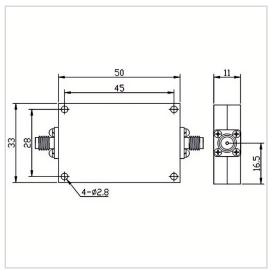
RF Solution offer a wide selection of High Pass Filter for global customers. HPF-3G12.75A-S is a High Pass Filter in Frequency Range of 3.0~12.75 GHz. It is made of high quality materials under a high standard, the Insertion Loss Max of this product is 1.5 dB, Rejection Min is 40dB@DC-2.7GHz and VSWR Max is 2.00. The component has a good working performance and stability, it is ideal for handling a Rated Power of 30 W.
