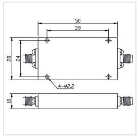
RF Solution offer a wide selection of High Pass Filter for global customers. HPF-2G18A-S is a High Pass Filter in Frequency Range of 2.0~18.0 GHz. It is made of high quality materials under a high standard, the Insertion Loss Max of this product is 2.0dB@2000-2250MHz / 1.0dB@2250-18000MHz, Rejection Min is 45dB@DC-1800MHz and VSWR Max is 1.80. The component has a good working performance and stability, it is ideal for handling a Rated Power of 20 W.
