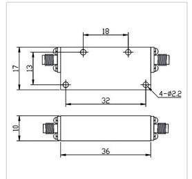
RF Solution offer a wide selection of High Pass Filter for global customers. HPF-2.5G18A-S is a High Pass Filter in Frequency Range of 2.5~18.0 GHz. It is made of high quality materials under a high standard, the Insertion Loss Max of this product is 1.5 dB, Rejection Min is 40dB@DC-2000MHz and VSWR Max is 1.60. The component has a good working performance and stability, it is ideal for handling a Rated Power of 15 W.
