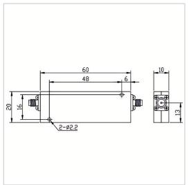
RF Solution offer a wide selection of High Pass Filter for global customers. HPF-1G18A-S is a High Pass Filter in Frequency Range of 1.0~18.0 GHz. It is made of high quality materials under a high standard, the Insertion Loss Max of this product is 2.00 dB, Rejection Min is 60dB min@DC-800MHz and VSWR Max is 2.00. The component has a good working performance and stability, it is ideal for handling a Rated Power of 10 W.
