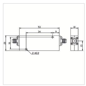
RF Solution offer a wide selection of High Pass Filter for global customers. HPF-1.6G12.75A-S is a High Pass Filter in Frequency Range of 1.6~12.75 GHz. It is made of high quality materials under a high standard, the Insertion Loss Max of this product is 1.5 dB, Rejection Min is 40dB@DC-1100MHz and VSWR Max is 1.80. The component has a good working performance and stability, it is ideal for handling a Rated Power of 30 W.
