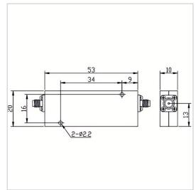
RF Solution offer a wide selection of High Pass Filter for global customers. HPF-1.2G13A-S is a High Pass Filter in Frequency Range of 1.2~13.0 GHz. It is made of high quality materials under a high standard, the Insertion Loss Max of this product is 2.00 dB, Rejection Min is 40dB@DC-960-1010MHz / 50dB@DC-960MHz and VSWR Max is 2.00. The component has a good working performance and stability, it is ideal for handling a Rated Power of 20 W.
