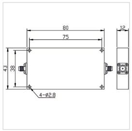
RF Solution offer a wide selection of High Pass Filter for global customers. HPF-1.1G9A-S is a High Pass Filter in Frequency Range of 1100~9000 MHz. It is made of high quality materials under a high standard, the Insertion Loss Max of this product is 3.00 dB, Rejection Min is 60dB min@DC-946MHz and VSWR Max is 2.00. The component has a good working performance and stability, it is ideal for handling a Rated Power of 20 W.
