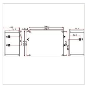
RF Solution offer a wide selection of RF Duplexer for global customers. DUP-412M422-05S is a RF Duplexer in Frequency Range of 412~427 MHz. It is made of high quality materials under a high standard, the Insertion Loss Max of this product is 1.7 dB, Ripple Max is 1.0 dB and Return Loss Min is 18 dB. The component has a good working performance and stability, it is ideal for handling a Average Power of 50 W.
