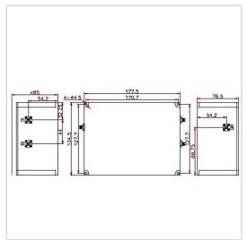
RF Solution offer a wide selection of RF Duplexer for global customers. DUP-385M395-05S is a RF Duplexer in Frequency Range of 385~400 MHz. It is made of high quality materials under a high standard, the Insertion Loss Max of this product is 1.7 dB, Ripple Max is 1.0 dB and Return Loss Min is 18 dB. The component has a good working performance and stability, it is ideal for handling a Average Power of 50 W.
