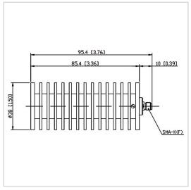
RF Solution offer a wide selection of Coaxial Fixed Termination (Dummy Load) for global customers. CT-50W-RA3885-SK-12.4G is Coaxial Termination (Dummy Load) in Frequency Range of DC~12.4 GHz. It is made of high quality materials under a high standard, the Connector Type of this product is SMA-F (K), VSWR Max is 1.35 and Impedance is 50  $\Omega$ . The component has a good working performance and stability, it is ideal for handling a Power of 50 W.
