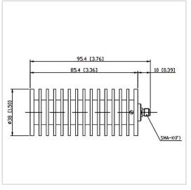
RF Solution offer a wide selection of Coaxial Fixed Termination (Dummy Load) for global customers. CT-50W-RA3885-SK-10G is a Coaxial Fixed Termination (Dummy Load) in Frequency Range of DC~10.0 GHz. It is made of high quality materials under a high standard, the Connector Type of this product is SMA-F (K), VSWR Max is 1.30 and Impedance is 50  $\Omega$ . The component has a good working performance and stability, it is ideal for handling a Power of 50 W.
